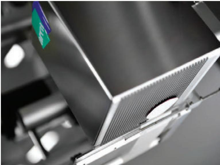
*With the Air Jet, labeler and product are never in contact and the adaptation is carried out by air blast. Product stabilizing devices are not needed and the labeler can even be positioned perpendicularly to the line.*
